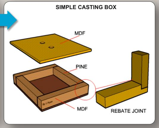
USING NOTES AND SKETCHES, DESCRIBE THE 'PACKING' OF THE BOX WITH SAND, READY FOR CASTING
