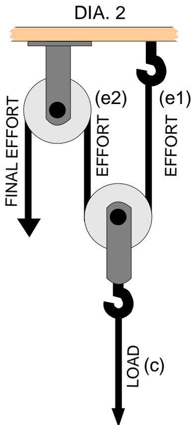
5. Why is a pulley system as seen in Dia. 2, easier to use than the one shown in Dia 1 (seen above)?
