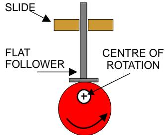
Opposite, is a simple diagram of an eccentric cam. I could use this design in my mechanical toy/game. Eccentric cams are easy to manufacture as the profile can be cut from a piece of large diameter dowel rod or even a floor brush handle.
