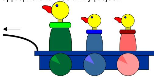
This mechanical toy is based on a cam mechanism. As the toy is pulled along the heads of the 'ducks' move up and down.
