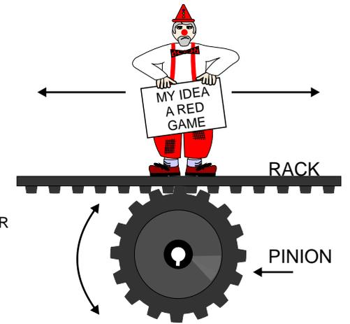
The rack and pinion gear system drawn above, could be applied to a mechanical toy/game. As the pinion gear wheel rotates in a clockwise direction, the rack gear moves to the right, and so does the model fixed to the top. If the pinion rotates anticlockwise the rack and model moves to the left.
