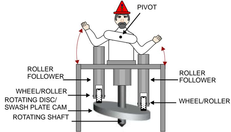
The mechanical display above is a dancing puppet. As the swash plate cam rotates the two roller followers rise and fall. This motion makes the puppet look as if it is dancing / waving its arms. The cam mechanism would normally be 'boxed in' for safety reasons.
