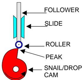
Snail/Drop cam. When rotating for one complete revolution the follower stays level for approximately the first 120 degrees. The follower then rises slowly and suddenly drops when it reaches and passes the peak. This is a useful cam if a sudden action is required. I could apply this cam to my mechanical toy.
