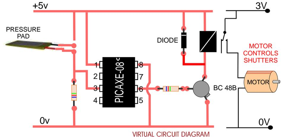
The circuit above shows how both input and output devices can be connected to the PICAXE-08.
