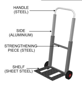
The trolley is manufactured from round section steel tube, solid section round steel, sheet steel, square section steel tube and square section aluminium tube.
