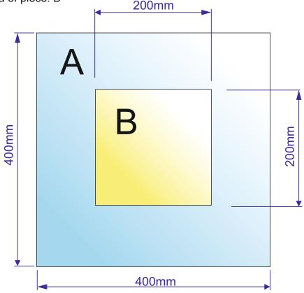
First, calculate the entire area of 'A', without the centre piece being removed, by treating it as a square 400mm x 400mm.
