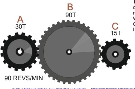
The diagram opposite shows a gear train composed of three gears. Gear A revolves at 90 revs/min in a clockwise direction.
