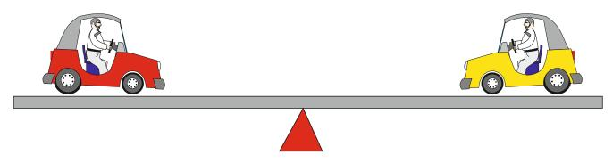
The cars are in a 'state of equilibrium' because the weight, on either side, is exactly the same. The distance from each car to the fulcrum, is also the same.
