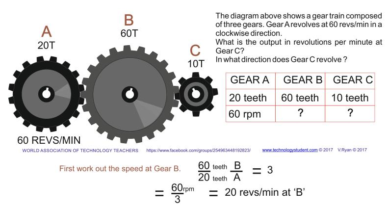
(Remember B is larger than A therefore, B outputs less revs/min and is slower)
