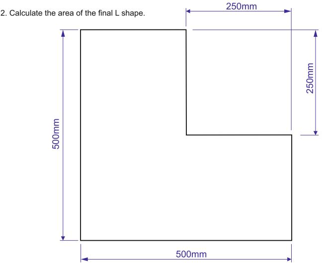
First, calculate the area of the uncut plywood, by treating it as a square 500mm x 500mm.
