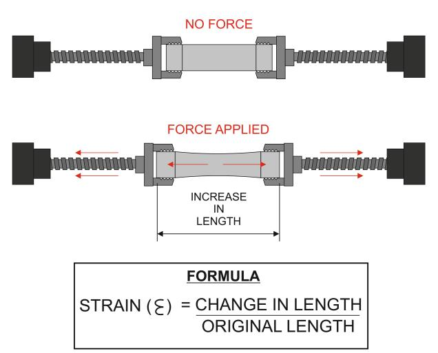
The sample metal (above) being tested, is 200mm in length when no force is applied (no load). However, when force / a load is applied it stretches to a length of 210mm. What is the 'strain'.
