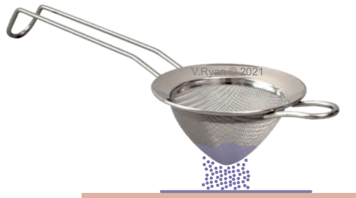
9. ENAMEL POWDER SIEVE THROUGH A MESH
